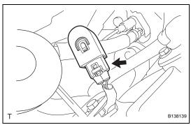
(b) Disconnect the connector and remove the wireless door lock buzzer.
